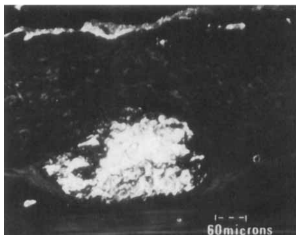
FIGURE 4 Illustration of 'contouring' behaviour round surface contamination
